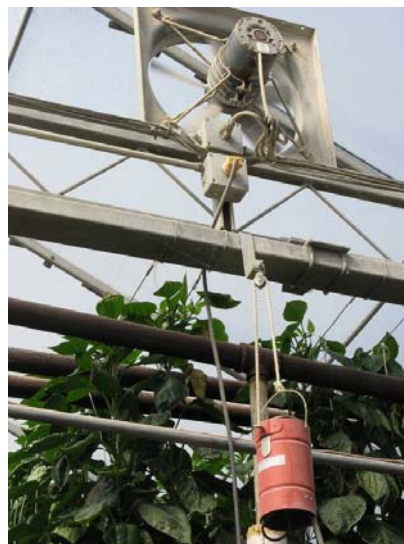
Trial Sulphur distribution system
